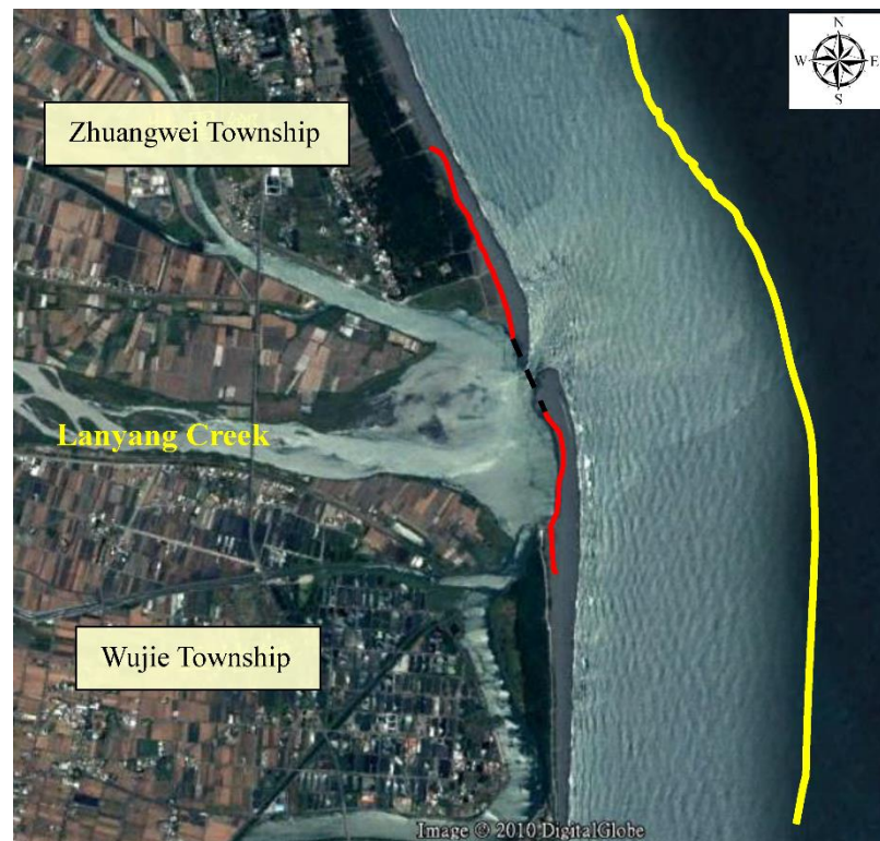
Figure 8. Preliminary planning results of coastal buffer zone using the SBEACH and wave run-up models (the estuary of Lanyang Creek, Yilan, Taiwan) [56]. (Red line: the onshore boundary of the coastal buffer zone; yellow line: the offshore boundary of the coastal buffer zone.).
