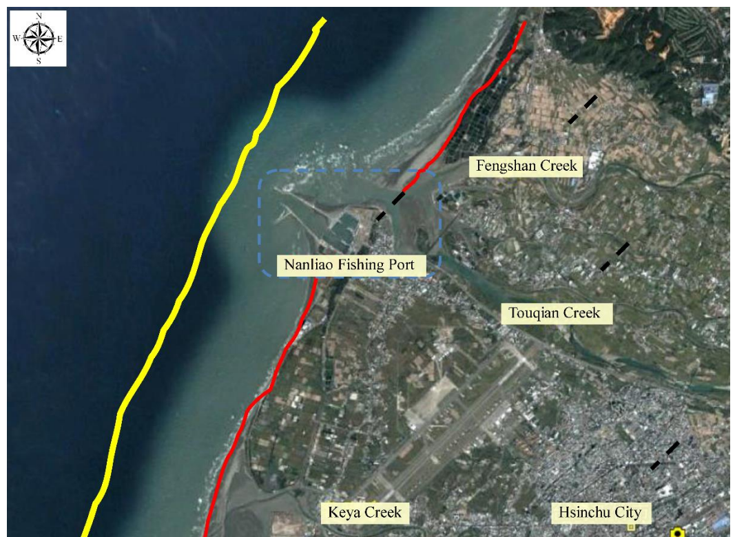
Figure 9. Preliminary planning results of coastal buffer zone using the SBEACH and wave run-up models (Nanliao Fishing Port, Hsinchu, Taiwan) [56]. (Red line: the onshore boundary of the coastal buffer zone; yellow line: the offshore boundary of the coastal buffer zone.).
